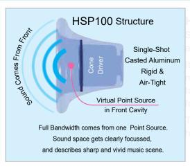
**HSP100**'s enclosure shape is designed to have a Virtual Point Source in the cavity in front of a Cone Driver. Audiences feel that all the sound is radiated from that one point.
